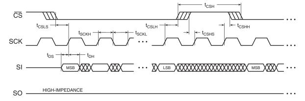
Figure 13-2. Serial Output Timing
