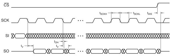
Figure 13-3. WP Timing for Write Status Register Command When SPRL = 1
